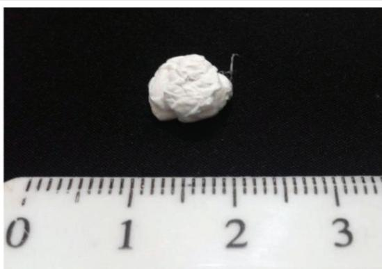
**Figure 4:** Image of dried BSM obtained by water substitution with ethanol followed by drying in laboratory oven at 50 °C.
