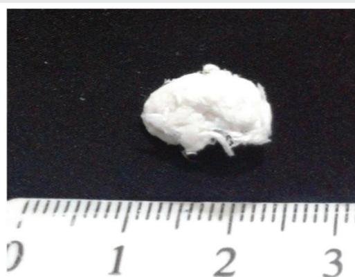
**Figure 6:** Image of dried BSM obtained by water substitution with ethanol followed by SC-CO<sub>2</sub> gel drying method.
