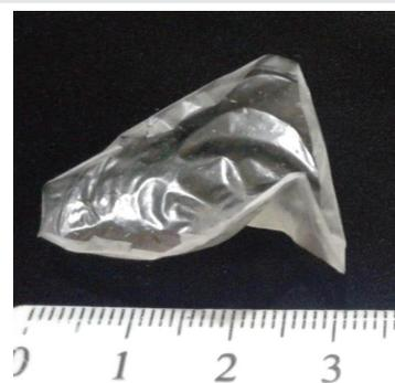
Figure 2: Image of dried BSM with air in a laboratory oven at 50 °C for 6 h.
